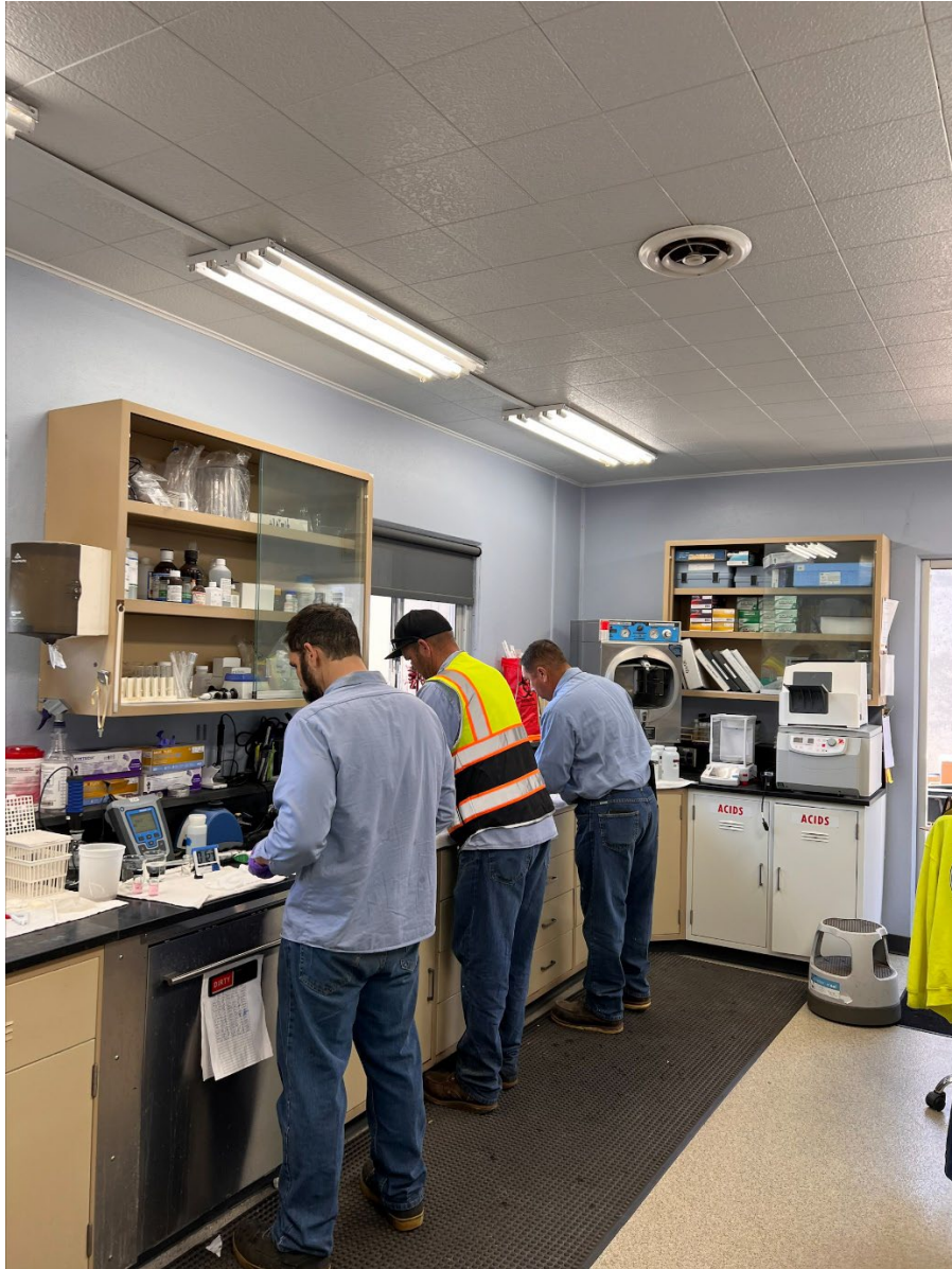
Operator in Training Robert Grajeda, Operator Justin Musick, and Operator in Training Everardo Vargas performing Demonstration of Capability (DOC) on Total Chlorine Residual analysis and pH analysis in the laboratory. DOC procedures are performed annually to establish the ability of the analyst to generate analytical results of acceptable accuracy and precision.
